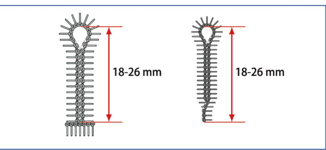
With -02-L1826 spec., one single machine sup-ports a wide range of applications, from straight-bartack buttonholes for casual pants to taper-bartack buttonholes for jeans. Sewing length of this spec. is 18-26 mm.
